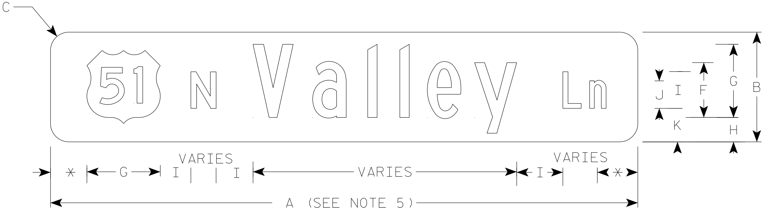
Typical for Overhead Street Name with Shield
