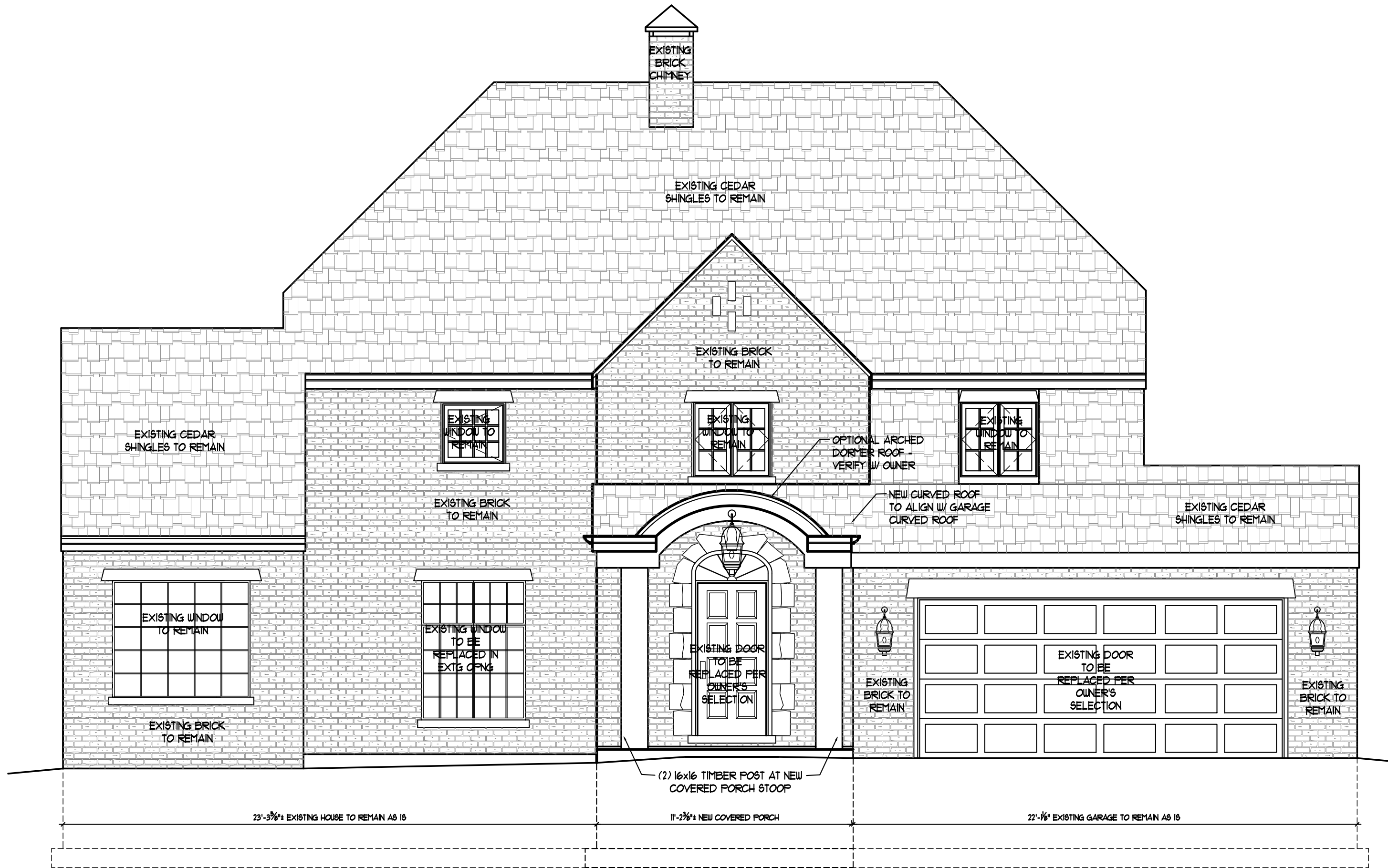
PROPOSED NEW COVERED PORCH EAST (STREET) ELEVATION SCALE: 1/4" = 1'-0"
