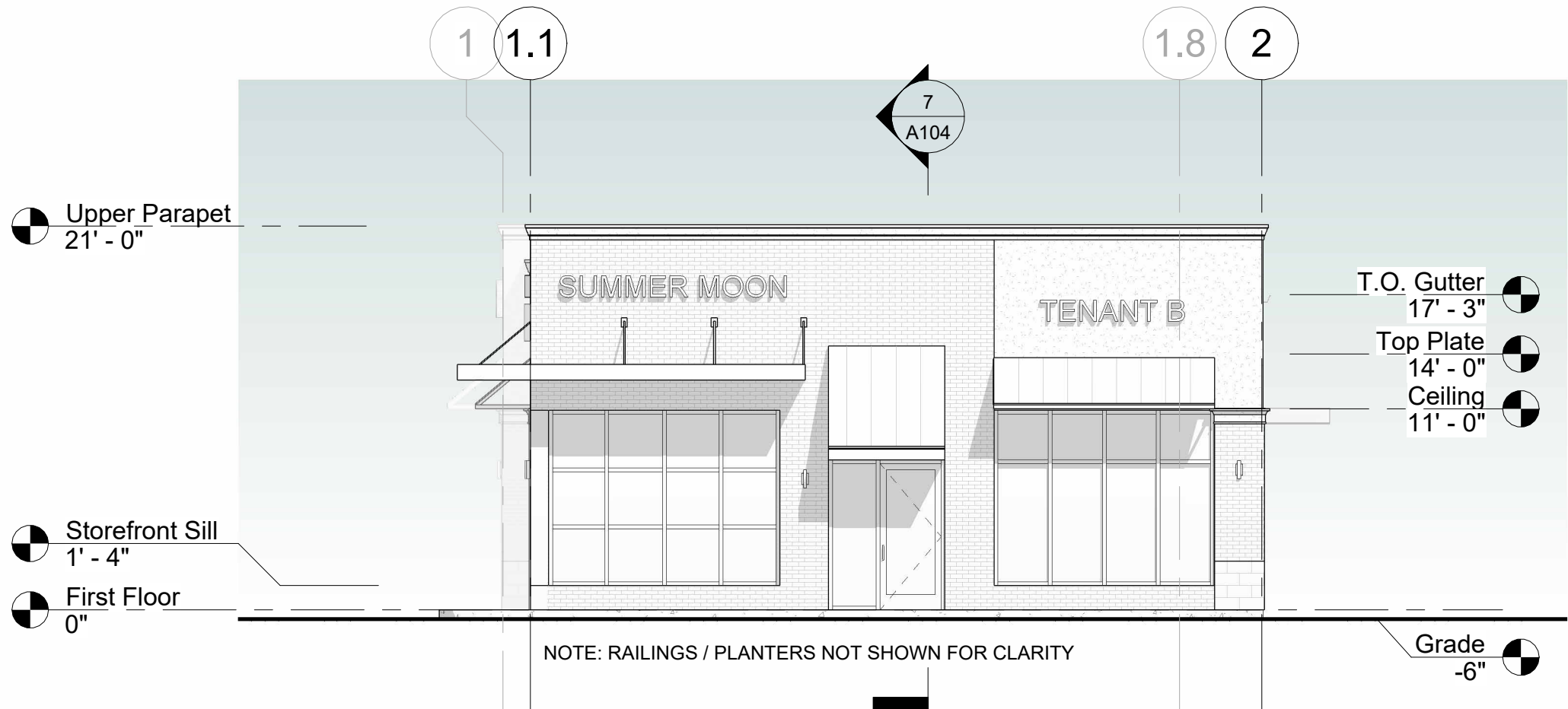
3 West Exterior Elevation 1/8" = 1'-0"
