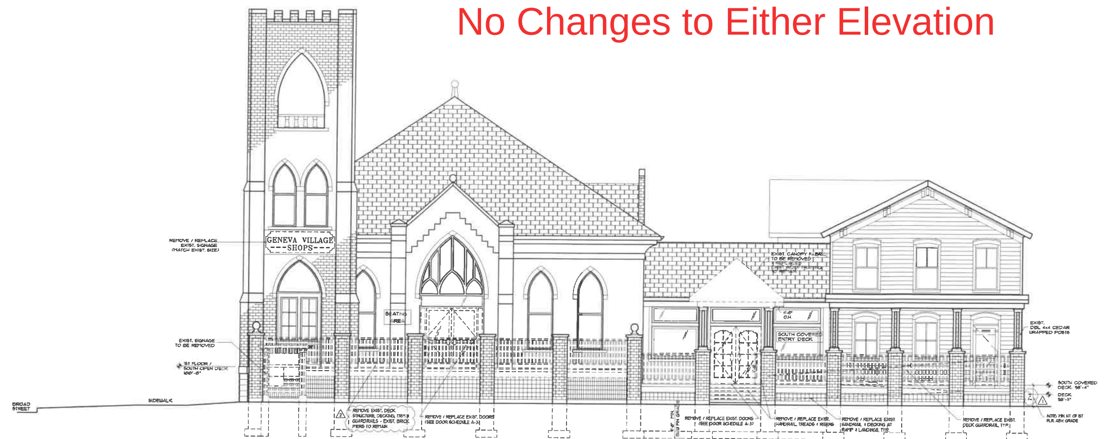
EXISTING - DEMOLITION SOUTH ELEVATION (GENEVA STREET) SCALE: 1/4" = 1'-0"
